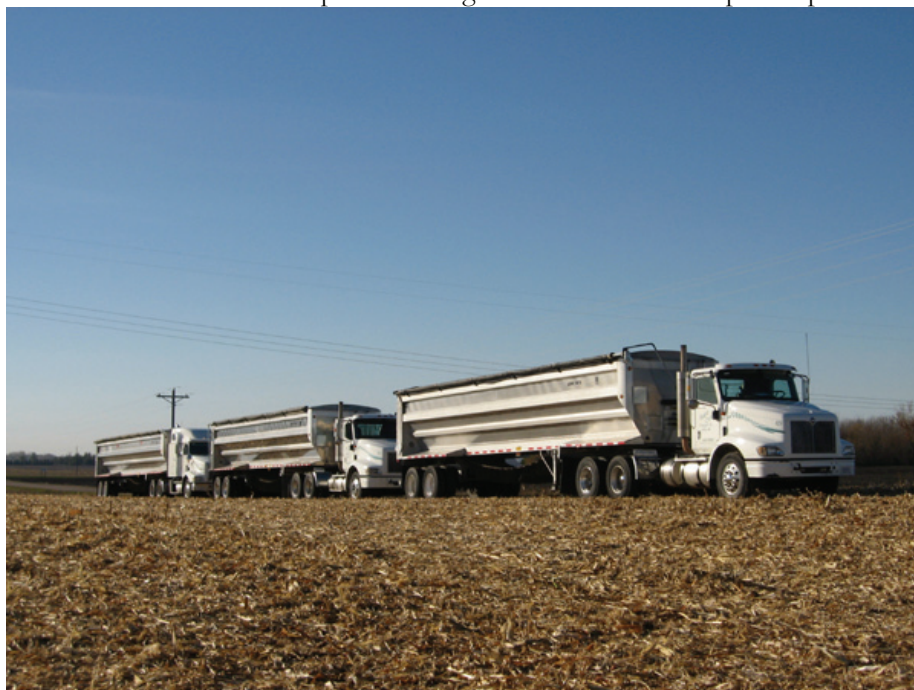
Beaver Creek Transport: Walking Floor Trailers with Open Tops
